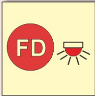
Space protected by automatic fire alarm
