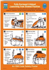
Fully Enclosed Lifeboat Launching from Stowed Position
