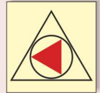
Remote control for fire pump(s)
