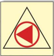
Remote control for emergency fire pump or fire
