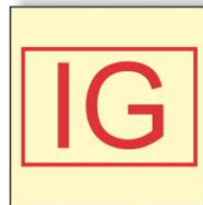
Intert gas installation
