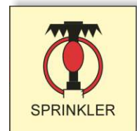
Space protected by sprinkler
